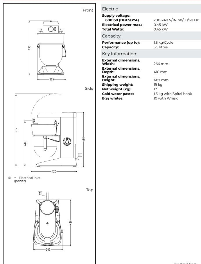
Planetary Mixers Planetary Mixer, 5 lt. - Electronic with Hub
